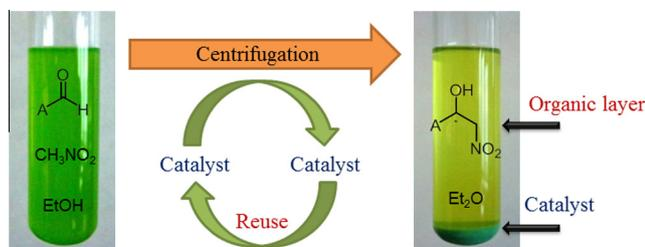
**Figure 4.** Principle of recycling of catalyst PEG-*b*-PG-CuL-1(2).
