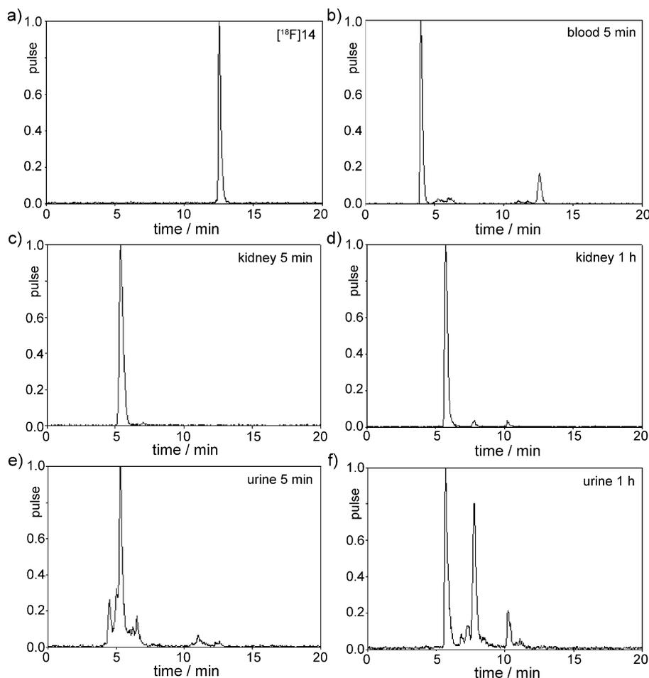
**Figure 5.** Representative HPLC traces of a) peptide  $[^{18}\text{F}]\mathbf{14}$  and determination of radioactive metabolites in b) arterial blood plasma; c, d) kidneys; and e, f) urine following single intravenous injection into a Wistar rat, determined 5 min and 1 h post-injection, as indicated.
