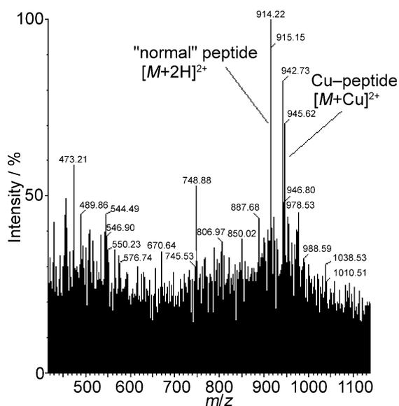
**Figure 2.** Part of the mass spectrum of **7** prepared in solution, indicating the formation of the Cu-peptide species.
