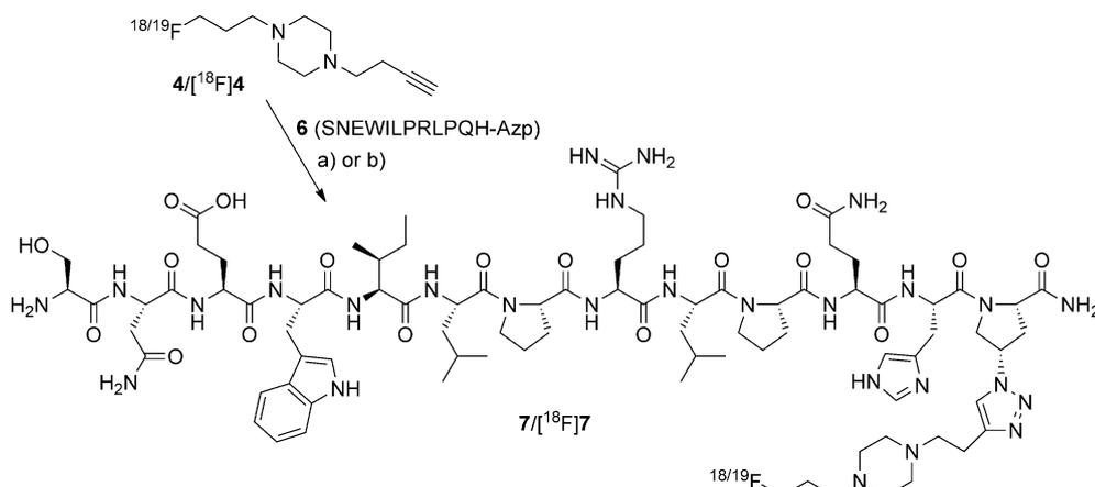
**Scheme 2.** Synthetic pathway to  $^{18/19}\text{F}$ -containing SNEW peptides **7**/[ $^{18}\text{F}$ ]**7** radiolabeled with [ $^{18/19}\text{F}$ ]BFP **4**/[ $^{18}\text{F}$ ]**4**. Reagents and conditions: a) DMF, sodium ascorbate, CuSO<sub>4</sub>·5H<sub>2</sub>O, 40 °C, 16 h; radiolabeling: b) DMF/Sørensen phosphate buffer, TBTA, sodium ascorbate, CuSO<sub>4</sub>·5H<sub>2</sub>O, 50 W, 1 h.
