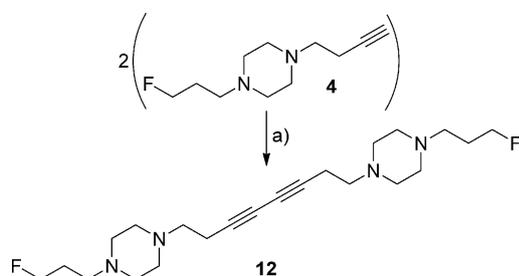
**Scheme 4.** Glaser coupling of BFP  $\mathbf{4}$  for the identification of byproduct  $\mathbf{12}$ . Reagents and conditions: a)  $\text{CuSO}_4 \cdot 5\text{H}_2\text{O}$ , DMF,  $40^\circ\text{C}$ , 3 days.
