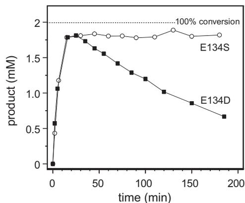
**Figure 2.** Time-course monitoring of the glycosynthase reactions catalyzed by the E134D and E134S mutants. Conditions: 2 mM Glc $\beta$ 4Glc $\beta$ 3Glc $\alpha$ F donor, 20 mM Glc $\beta$ pNP acceptor, 2  $\mu$ M enzyme, pH 7.0, 35 °C.
