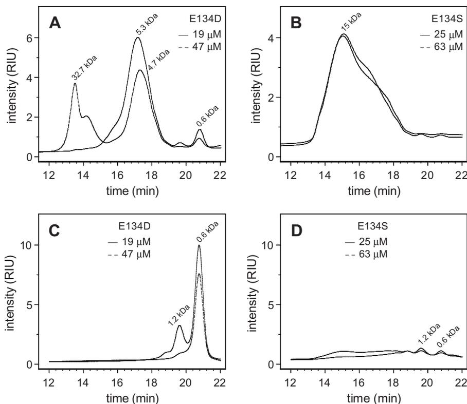
**Figure 6.** Size exclusion chromatograms (HPSEC) of the insoluble polysaccharides by glycosynthase-catalyzed polymerization, (A) with E134D, (B) with E134S, and of the soluble fractions, (C) with E134D, (D) with E134S, at two different enzyme concentrations. Mp values (maximum of the peaks) are indicated in kDa.
