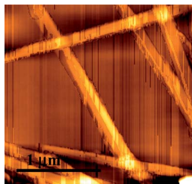
Fig. 7 AFM image of aggregates obtained from {Fmoc-(L)Glu + (L)Lys} in the presence of \text{Ca}^{2+} ions.
