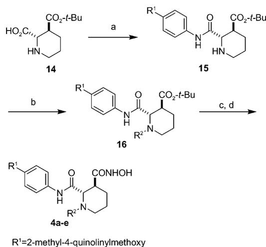
**Scheme 3.** Reagents and conditions: (a) 4-[(2-methyl-4-quinolinyl)methoxy]aniline, BOP, DIEA, DMF, 68%; (b) aldehyde, Na(OAc)<sub>3</sub>BH, DIEA, THF; (c) TFA, CH<sub>2</sub>Cl<sub>2</sub>; (d) hydroxylamine hydrochloride, BOP, DIEA, DMF.
