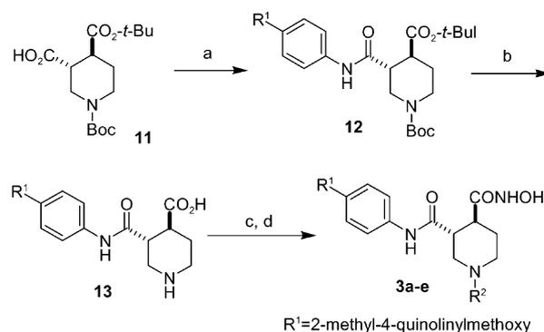
**Scheme 2.** Reagents and conditions: (a) 4-[(2-methyl-4-quinolinyl)methoxy]aniline, BOP, DIEA, DMF, 78%; (b) TFA, CH<sub>2</sub>Cl<sub>2</sub>, 100%; (c) an aldehyde, Na(OAc)<sub>3</sub>BH, DIEA, THF or 2-furoyl chloride, NMM, THF, H<sub>2</sub>O; (d) hydroxylamine hydrochloride, DIEA, BOP, DMF.
