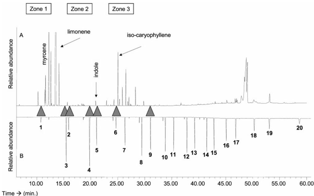
**Figure 1.** (A) GC-TIC trace on apolar column of the crude extract. (B) Inverted GC-TIC trace of an equimolar mixture of synthetic thiols from 1 to 20. Marks represent retention times where sulfury odors were smelled.
