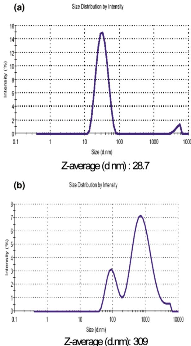
**FIGURE 5.** Hydrodynamic diameter of colloidal gold particles as measured by dynamic light scattering system (a) before enhancement and (b) after enhancement treatment with a solution of 0.01% gold chloride in 0.4 mM hydroxylamine for 2 min at RT.
