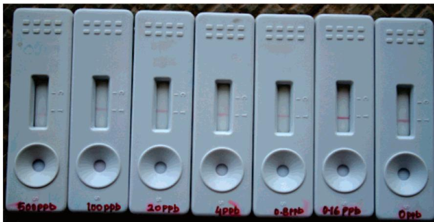
**FIGURE 10.** Sensitivity of immunochromatographic dipstick for atrazine samples. Samples spiked with different concentrations of atrazine were added to the sample well and the response was recorded using a digital color camera after 3 min of sample addition.
