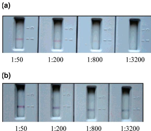
**FIGURE 6.** Effect of gold-enhancer on improvement of visibility of color of test line on NC membrane (a) before and (b) after enhancement. Tracer dilutions (1:50; 1:200; 1:800, and 1:3200) were prepared in PBS.
