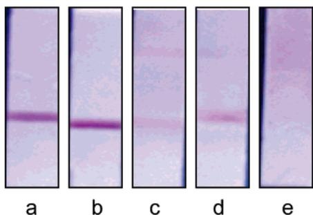
**FIGURE 4.** Effect of various buffers on antibody coating on dipstick membrane: (a) 50 mmol phosphate, pH 7.2; (b) 50 mmol phosphate + 3% methanol, pH 7.2; (c) phosphate buffer saline, pH 7.2; (d) phosphate buffer saline + 3% methanol, pH 7.2; (e) 50 mmol phosphate + 150 mmol NaCl, pH 7.2. All samples were detected by a 40 nmol gold-hapten conjugated BSA.
