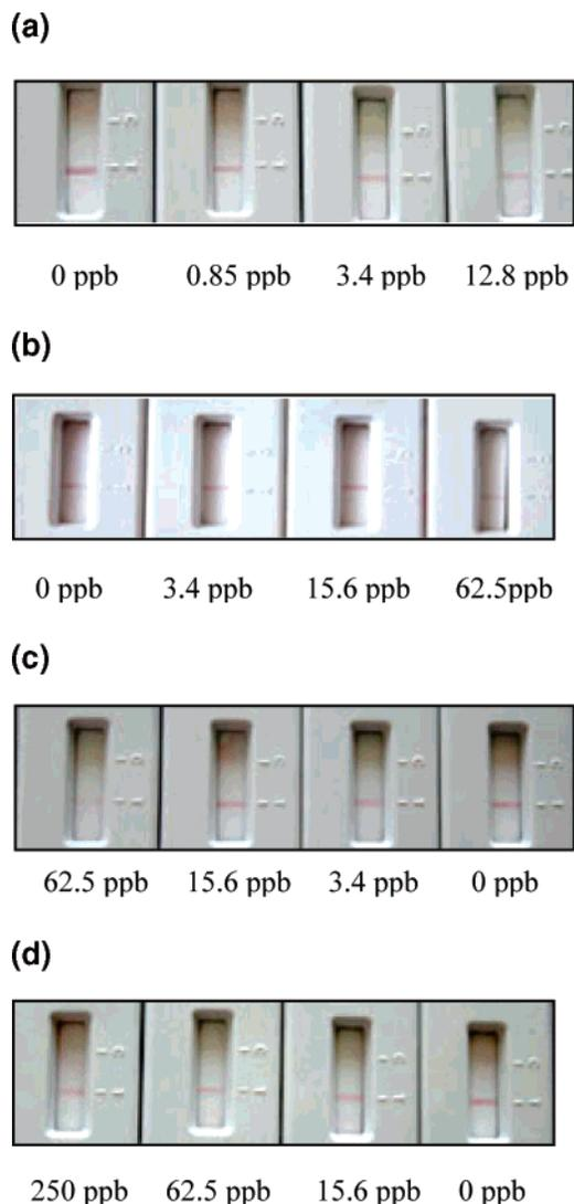
**FIGURE 9. Cross-reactivity of immunochromatographic dipstick coated with anti-atrazine antibody with atrazine and its analogues: (a) atrazine, (b) simazin, (c) prometon, and (d) terbutryn. Stock solutions of samples were prepared in methanol (1 mg/mL) and further diluted in PBS buffer for assay.**
