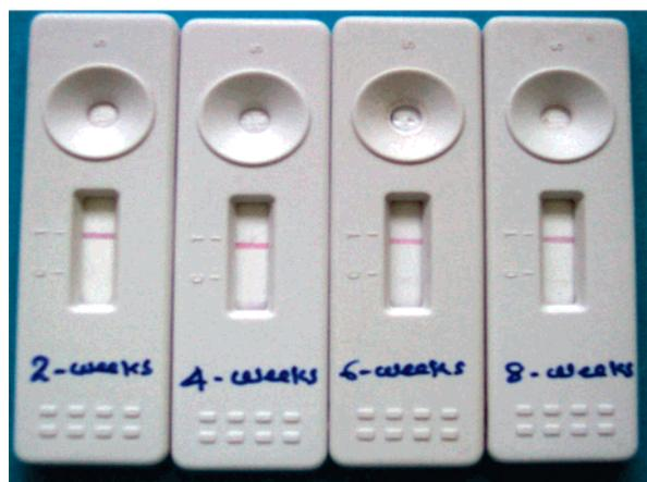
**FIGURE 11.** Stability test of developed gold–protein–hapten conjugate. The dipsticks were subjected to tracer solution (hapten–gold–protein conjugate) after 2, 4, 6, and 8 weeks of their storage in ambient conditions (room temperature in a desiccator).
