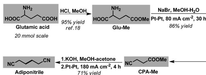
Figure 2. Full process for synthesis of adiponitrile.
