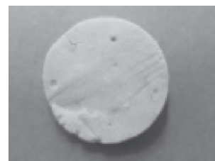
Fig. 8. Photograph of sample of PEA 80/20S after 98 days of immersion in phosphate buffer.
