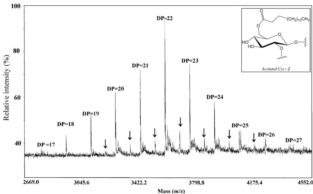
**Figure 10.** MALDI-TOF MS containing acylated Cys-2. The arrows are the intermediates corresponding to the acylated Cys-2. The arrows indicate the intermediates formed on Cys, of which the measured masses are observed as  $m/z$  3200, 3361, 3523, 3686, 3847, 4009, and 4172, respectively. These sequential ions corresponded to the [acylated Cys-2<sup>+</sup> + 2Na<sup>+</sup> +  $n$ H<sup>+</sup>] ( $n = -1$  or 0). Inset indicates a possible acylated Cys-2.
