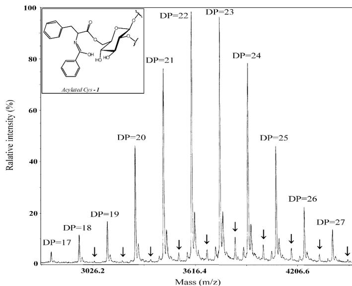
**Figure 5.** MALDI-TOF MS containing acylated Cys-1. The arrows are the intermediates corresponding to the acylated Cys-1. The arrows indicate the intermediates formed on Cys, of which the measured masses are observed as  $m/z$  3035, 3197, 3359, 3521, 3684, 3846, 4008, 4170, 4332, and 4494, respectively. These sequential ions represent the  $[\text{acylated Cys-1}^+ + \text{Na}^+ + 9\text{H}^+]$ . The inset indicates a possible acylated Cys-1.
