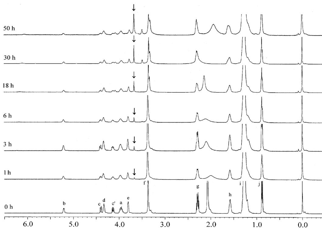
**Figure 7.** <sup>1</sup>H NMR spectra for methanolysis of **2** catalyzed by Cys with increasing reaction time. The arrows indicate the resonances of methoxy protons of methyl palmitate made from methanolysis of **2** catalyzed by Cys.
