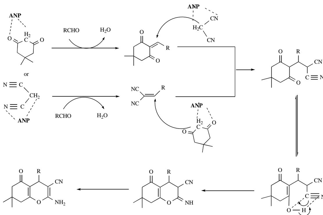
**Scheme 2.** A possible mechanism of ANP-catalyzed Hantzsch reaction.
