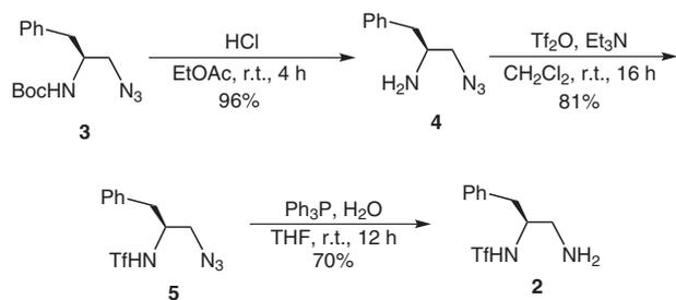
**Scheme 2** Preparation of the organocatalyst
