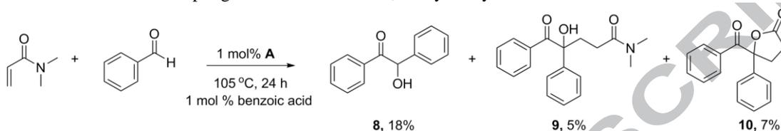
**Scheme 6.** The reaction of benzaldehyde and DMAA catalyzed by NHC A.
