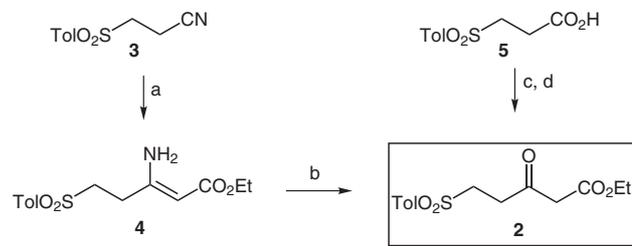
**Scheme 1** Reagents and conditions: (a) Zn, BrCH<sub>2</sub>CO<sub>2</sub>Et, MsOH, THF, reflux, 3 h; (b) HCl, THF, r.t., 2 h, 75% from **3**; (c) 1,1'-carbonyldiimidazole, THF, r.t., 4 h; (d) HO<sub>2</sub>C(CH<sub>2</sub>)CO<sub>2</sub>Et, Mg(OEt)<sub>2</sub>, THF, r.t., 12 h, 80% from **5**.
