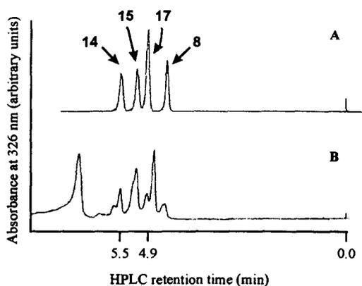
**Figure 1.** Typical HPLC chromatograms from the reductively triggered drug release study. A: Synthetic standards; B: **15** + Zn / NH<sub>4</sub>Cl (24 h).
