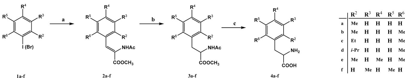
Reagents and conditions: a) methyl acetamidoacrylate, Pd(OAc)<sub>2</sub>, tri-*o*-tolylphosphine, Et<sub>3</sub>N, CH<sub>3</sub>CN, reflux 10 h; b) H<sub>2</sub> (60 psig), [Rh(1,5-COD)(*R,R*-DIPAMP)]BF<sub>4</sub>, 60 °C, 12 h; c) 12 mol/l HCl conducted under reflux conditions for 6 h.
