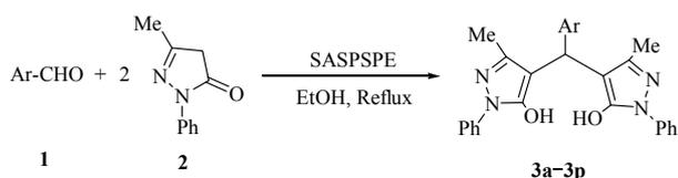
**Scheme 2.** The condensation of aromatic aldehydes with 3-methyl-1-phenyl-5-pyrazolone upon catalysis by SASPSPE.
