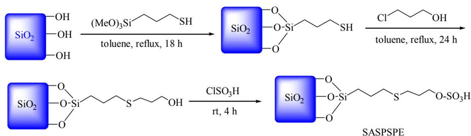
**Scheme 1.** Preparation of sulfuric acid ([3-(3-silicapropyl)sulfanyl]propyl)ester (SASPSPE).
