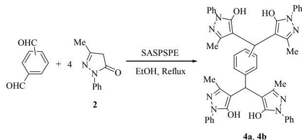
**Scheme 3.** The condensation of terephthalaldehyde with 3-methyl-1-phenyl-5-pyrazolone catalyzed by SASPSPE.
