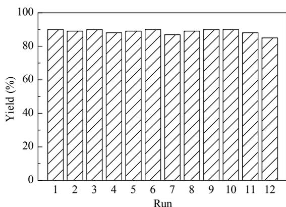
**Fig. 1.** Recyclability of SASPSPE as a catalyst in the condensation reaction between benzaldehyde (1 mmol) and 5-methyl-2-phenyl-2,4-dihydro-3H-pyrazol-3-one (2 mmol) in the presence of 0.1 g of SASPSPE in refluxing ethanol. Reaction time 3 h.
