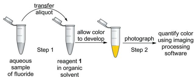
**Fig. 2** Schematic of the assay procedure for detecting fluoride colorimetrically. Step 1 involves diluting a sample that contains aqueous fluoride into a solution of **1**. After a period of time required for the autoinductive signal amplification reaction to proceed, photographs are taken (step 2) and the colorimetric response is measured using image-processing software.
