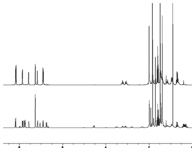
Fig. 3  $^1\text{H}$  NMR monitoring of the reaction between  $\text{AlEt}_3$  and **1a** (1:1 molar ratio,  $\text{C}_6\text{D}_6$ , 300 MHz, 297 K): after 2 hours of reaction at room temperature (bottom) and after 24 hours of heating at 40 °C (top).
