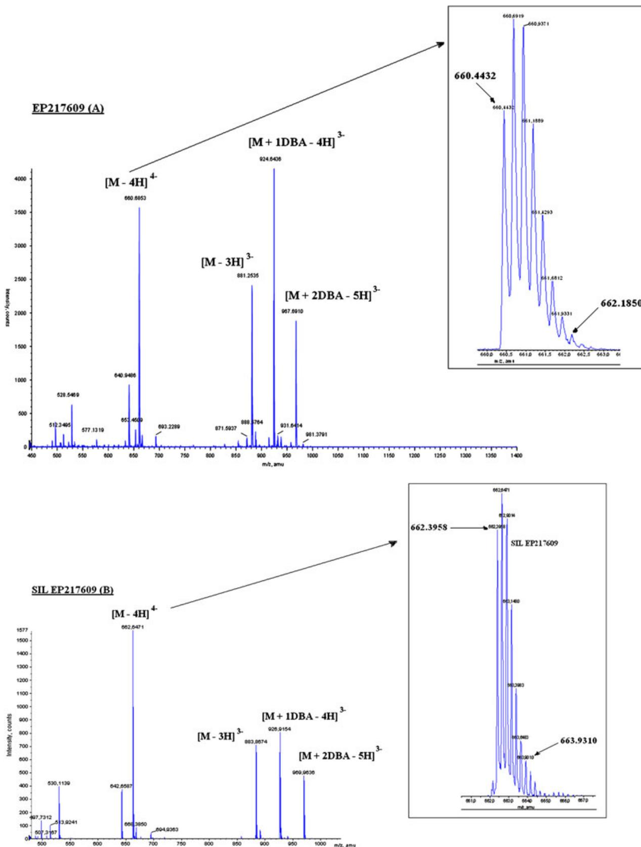
**Figure 2.** ESI-MS spectra of unlabeled (A) and labeled EP217609 (B) with an example of expanded region of molecular ion  $m/z$   $[M - 4H]^{4-}$  showing peaks from 660.4432 to 662.1850 for unlabeled compound (A) and peaks from 662.3958 to 664.1537 for labeled compound (B). DBA, dibutylamine.
