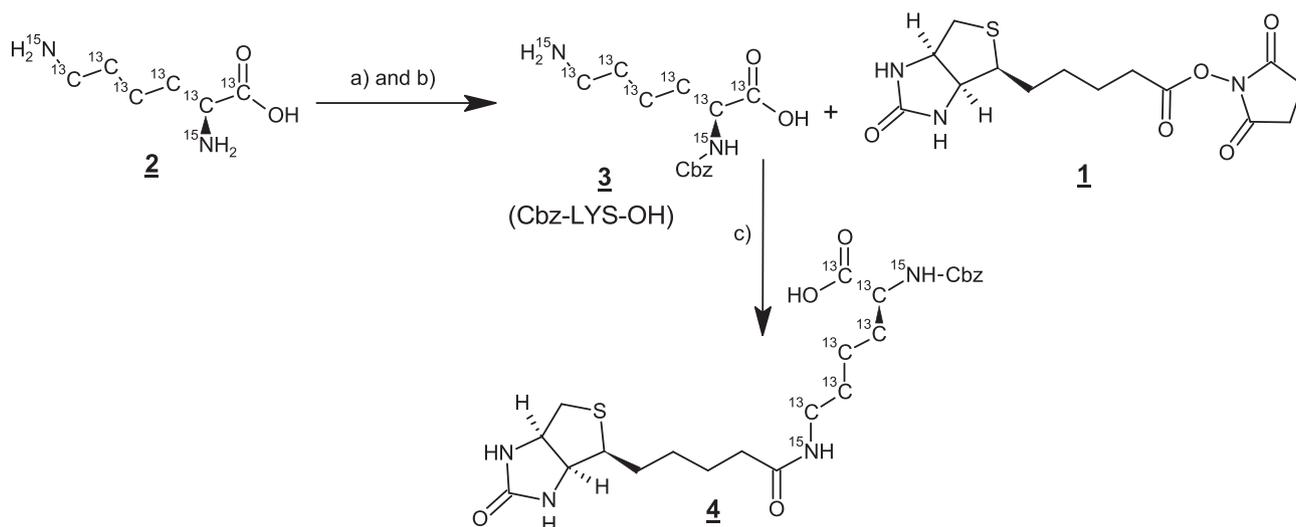
**Scheme 2.** (a) *p*-Anisaldehyde, 2N LiOH, 4 °C, overnight, not isolated; (b) 1N NaOH/EtOH, Cbz-Cl, -20 °C to -5 °C, conc. HCl, 78% over a and b; (c) DIEA, DMF, 95%.
