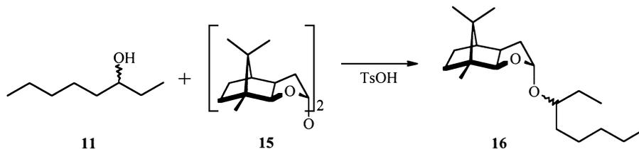
Scheme 3. Acetal formation of 3-octanol **11** with the anhydrolactol **15** for determination of the enantiomeric excess of **11** by GC
