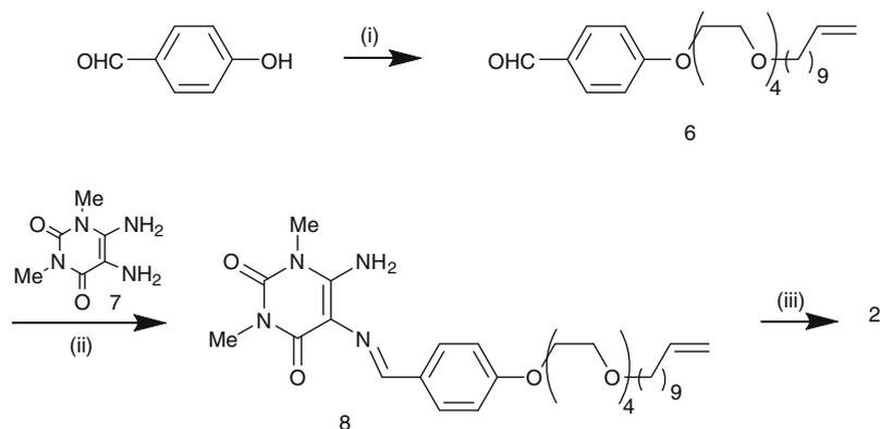
(i) 4,  $K_2CO_3/CH_3CN$ , reflux, 1h. (ii) 7, EtOH/AcOH, reflux, 12h. (iii) DIAD, DME, reflux, 12h.
