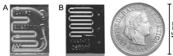
Figure 1. DeanFlow (A) and KombiMix (B) microreactor chips.
