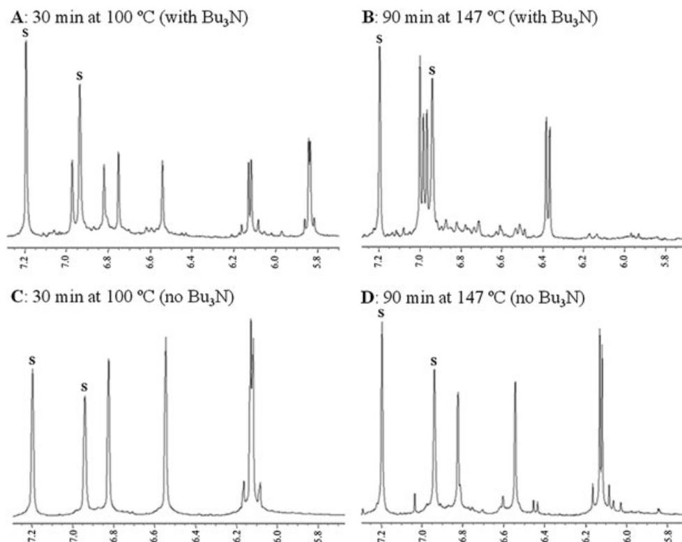
**Figure 1.**  $^1\text{H}$  NMR spectra (400 MHz; 7.2–5.8 ppm) from solutions isocyanate *E*-5 in  $d_r$ -dichlorobenzene after heating with (A and B) and without (C and D) tributylamine. Solvent peaks (S) are labeled (7.20 and 6.94 ppm).
