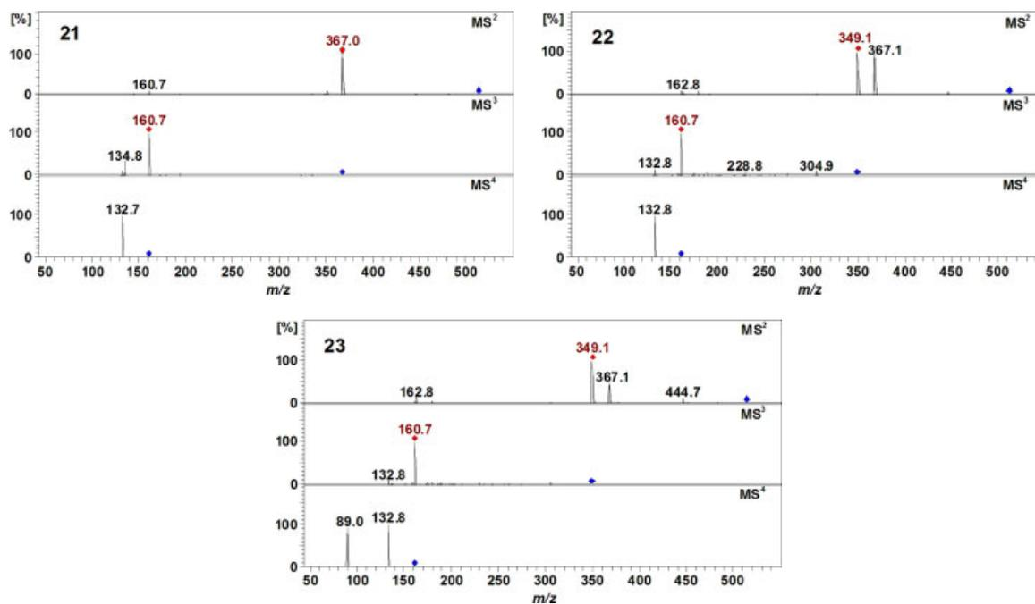
Figure 14. MS<sup>3</sup> spectra of methyl *p*-coumaroyl-caffeoylquinates (21–23) (parent ion at *m/z* 513 in negative ion mode).
