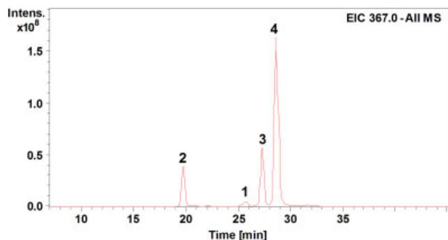
**Figure 3.** Extracted ion chromatogram (EIC) of methyl-caffeoylquinic acids (1–4) in negative ion mode at  $m/z$  367.
