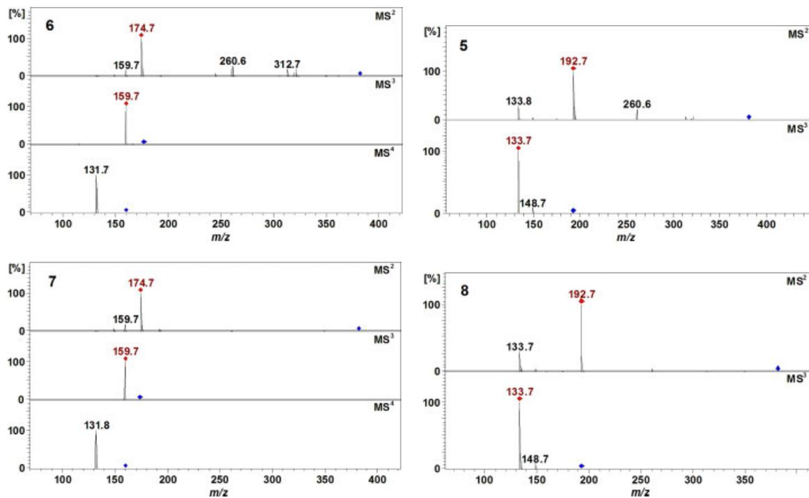
**Figure 7.** MS<sup>3</sup> spectra of methyl feruloylquinates (5–8) (parent ion at  $m/z$  381 in negative ion mode).
