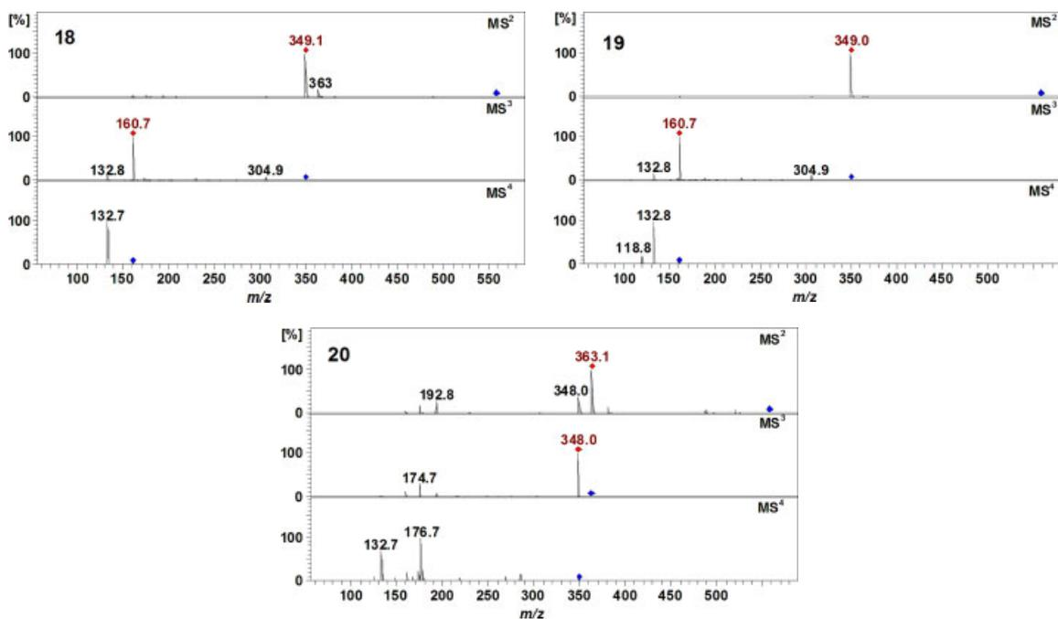
Figure 13. MS<sup>3</sup> spectra of methyl diferuloylquinates (18–20) (parent ion at *m/z* 557 in negative ion mode).
