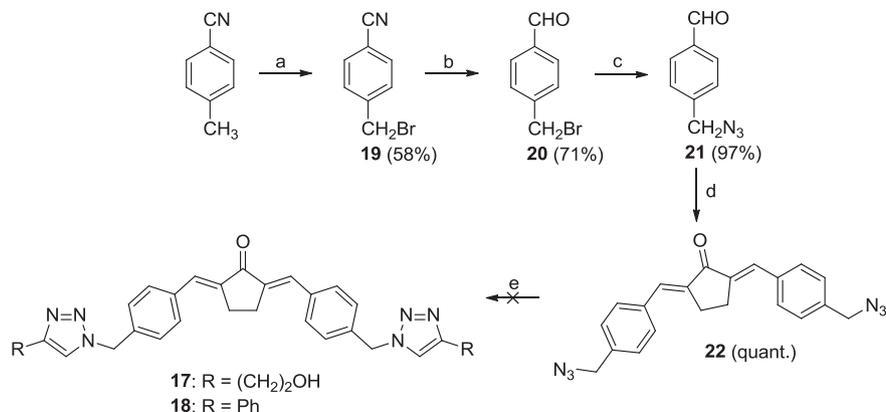
**Scheme 3.** Synthetic route for the preparation of compounds **17** and **18**. Reagents and conditions: (a) benzoyl peroxide, NBS, benzene, reflux, 4 h. (b) (i) DIBALH, toluene, 0 °C, N<sub>2</sub> atm, 2 h. (ii) HCl 10%, CHCl<sub>3</sub>, rt, 1 h. (c) NaN<sub>3</sub>, THF/water, reflux, 24 h. (d) NaOH 0.2 M, EtOH 95%, rt, 2 h. (e) Terminal alkyne, CuSO<sub>4</sub>·5H<sub>2</sub>O, sodium ascorbate, CH<sub>2</sub>Cl<sub>2</sub>/water, rt, 24 h.
