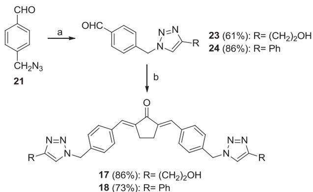
**Scheme 4.** Alternative route for the preparation of **17** and **18**. Reagents and conditions: (a) terminal alkyne, CuSO<sub>4</sub>·5H<sub>2</sub>O, sodium ascorbate, CH<sub>2</sub>Cl<sub>2</sub>/water, r.t., 24 h. (b) NaOH 0.2 M, EtOH 95%, r.t., 4–20 h.
