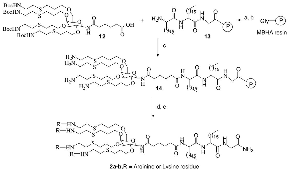
**Scheme 2.** Reagents and conditions: (a) i—2-amino-octadecanoic acid, HBTU, DIPEA, DMF, rt, 30 min; ii—TFA, rt, 2× 1 min; (b) i—2-Amino-octadecanoic acid, HBTU, DIPEA, DMF, rt, 30 min; ii—TFA, rt, 2× 1 min; (c) i—**12**, HBTU, DIPEA, DMF, rt, 30 min; ii—TFA, rt, 2× 1 min; (d) Boc-Lys(CIZ) (**2a**) or Boc-ArgTsOH (**2b**), HBTU, DIPEA, DMF, rt; ii—TFA, rt, 2× 1 min; (e) HF-cleavage.
