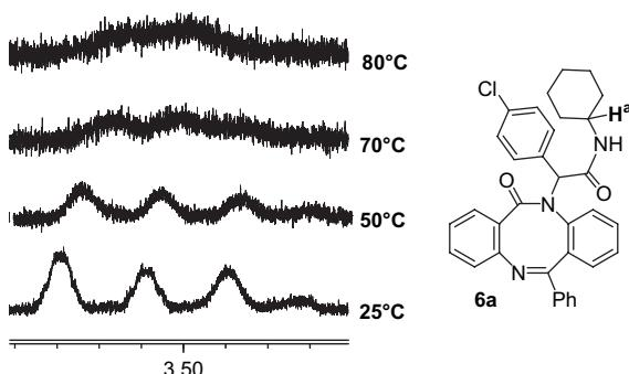
Figure 4.  $\text{H}^\alpha$  region of the  $^1\text{H}$  NMR spectra of **6a** in deuterated chlorobenzene at different temperatures.
