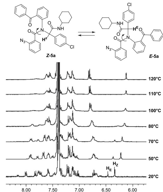
Figure 1. Selected region of <sup>1</sup>H NMR spectra of **5a** in deuterated chlorobenzene at different temperatures.
