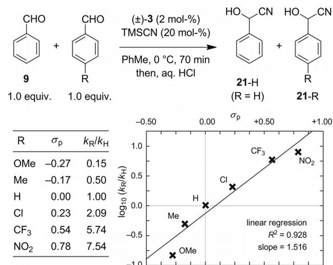
Figure 2. Hammett analysis of the competitive silylcyanation of 4-substituted benzaldehydes as compared with benzaldehyde.  $k_R/k_H$  is equal to the ratio of **21-R/21-H** and was determined by integration of the <sup>1</sup>H NMR spectrum of the crude product mixture.X-ray Diffraction Analysis of **3**
