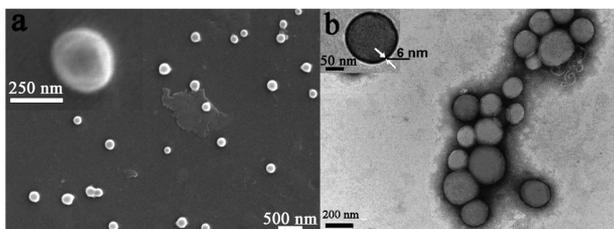
**Figure 2.** (a) SEM and (b) TEM images of the vesicles formed by amphiphile **1** in aqueous solution. Insets show the magnified photographs of the vesicle.
