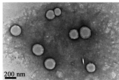
**Figure 3.** TEM image of the vesicles after polymerization.
