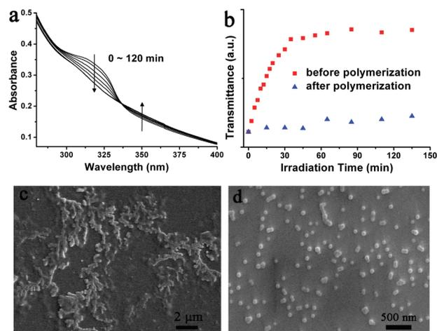
**Figure 4.** (a) Absorption spectra of polymeric vesicles upon UV irradiation. (b) Optical transmittance of different vesicle solutions as a function of UV irradiation time. SEM images of (c) unpolymerized vesicles and (d) polymeric vesicles after UV irradiation for 60 min.
