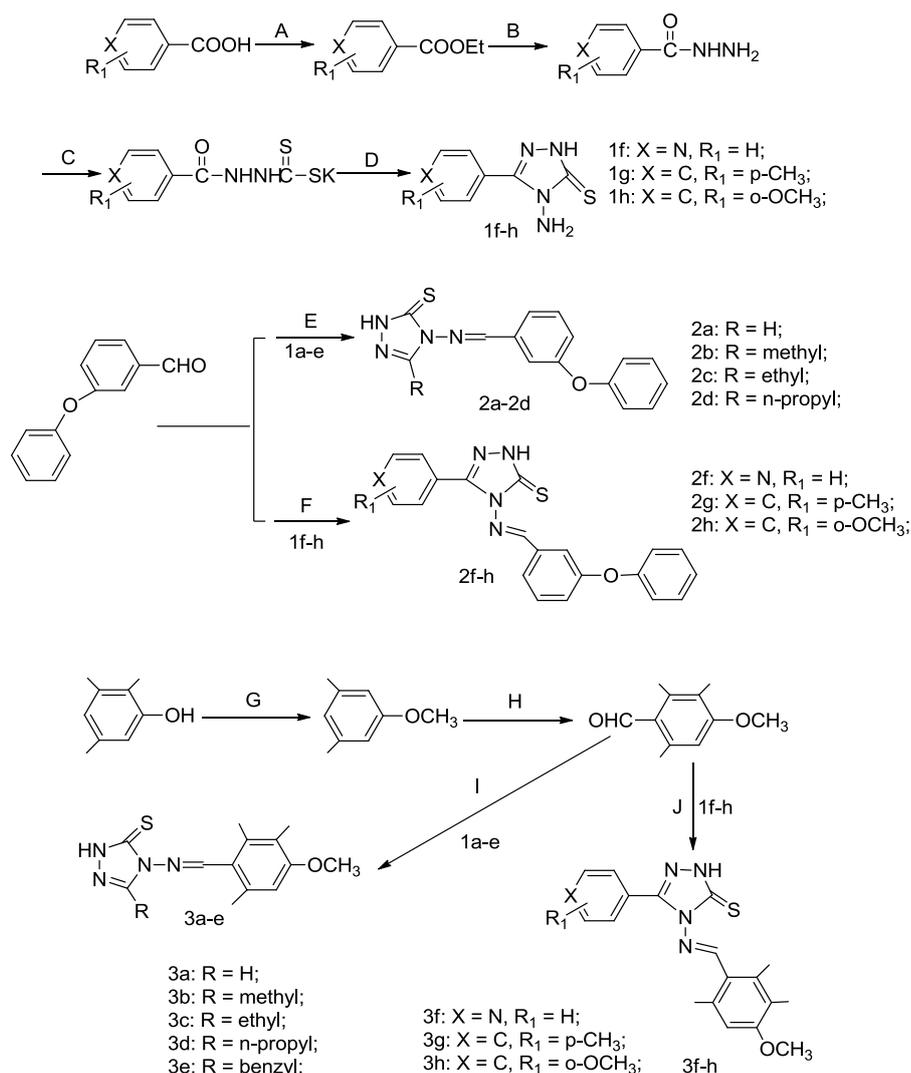
Scheme 1 Synthesis of 1,2,4-triazole Schiff bases. Reagents and conditions: (A) 98% H<sub>2</sub>SO<sub>4</sub>, EtOH, reflux; (B/D) NH<sub>2</sub>NH<sub>2</sub>·H<sub>2</sub>O, EtOH, reflux; (C) CS<sub>2</sub>, KOH, rt; (E/F/I/J) EtOH, CH<sub>3</sub>COOH, reflux; (G) CH<sub>3</sub>I, K<sub>2</sub>CO<sub>3</sub>, THF, reflux; (H) POCl<sub>3</sub>, DMF, NaOH, 90°C
