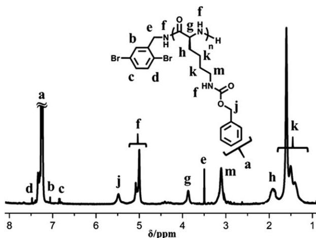
**FIGURE 2**  $^1\text{H-NMR}$  spectrum of polypeptide macromonomer, DBB-PLL.
