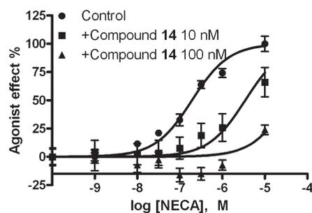
**Figure 5.** Antagonist activity of compound 14 in the stimulation of cyclic AMP accumulation induced by agonist NECA in CHO cells stably expressing the hA<sub>2B</sub>AR. Each curve is representative of three determinations. The EC<sub>50</sub> values for NECA in the absence and presence of 10 nM 14 are 194 nM and 3.46 μM, respectively.
