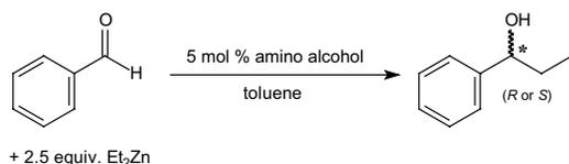
**Scheme 1.** Addition of diethylzinc to benzaldehyde catalyzed by chiral amino alcohols.
