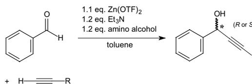
**Scheme 2.** Addition of phenylacetylene to benzaldehyde catalyzed by chiral amino alcohols.
