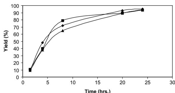
**Figure 4.** The effect of reaction time on the yield of 1-phenylpropanol using **P2** and regenerated **P2** in the addition of diethylzinc to benzaldehyde. Symbols: (◆) First run, (■) First regeneration, (▲) Second regeneration (entries 9–11 in Table 1).
