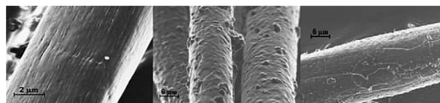
**Figure 5.** A scanning electron micrograph (SEM) of the unfunctionalized parent fiber **P0** (left) and the fibrous amino alcohol catalysts **P1** (middle) and **P2** (right).
