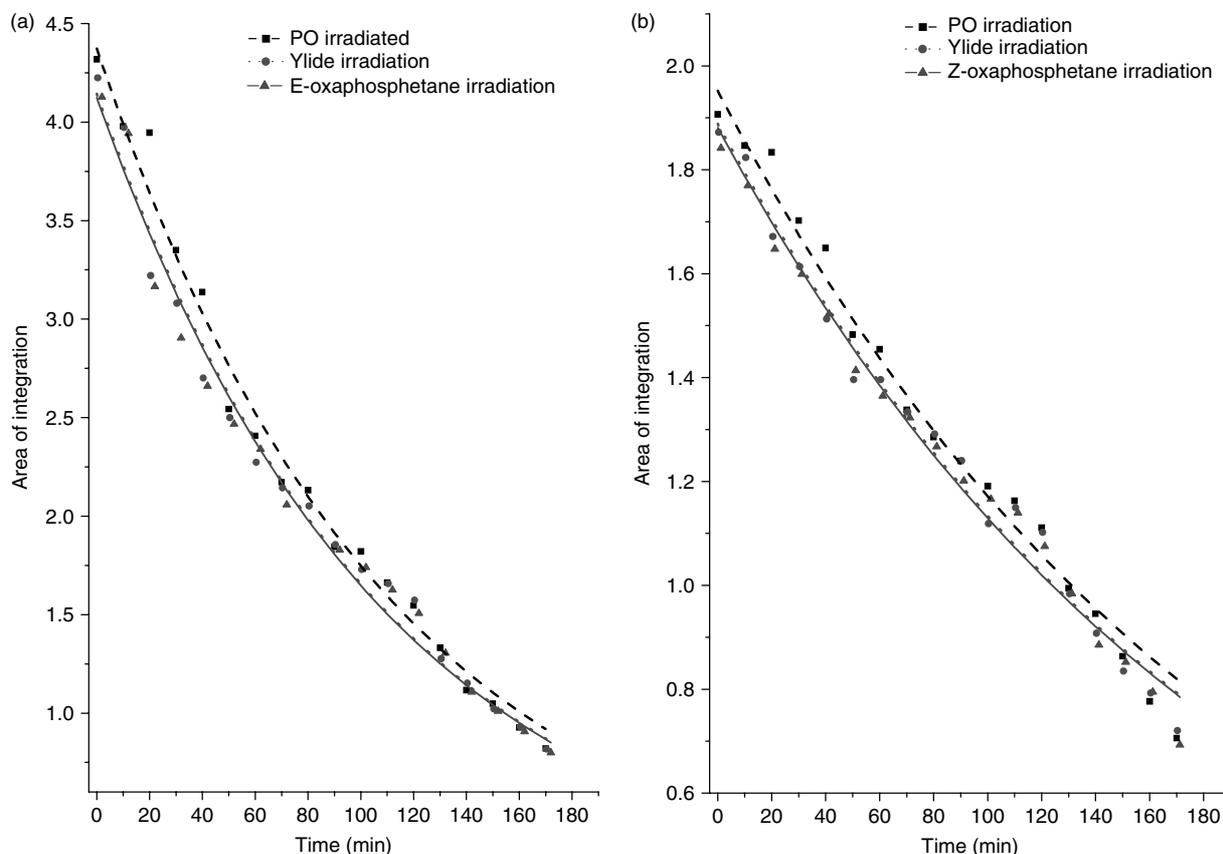
**Figure 3.** Time behaviour of the  $^{31}\text{P}$  NMR signals of the (a) (*Z*)- and (b) (*E*)-oxaphosphetane signals during the Wittig reaction at 253 K. The curves show the situation when the phosphane oxide signal was irradiated as a control (■) and the situation when the ylide signal (●) or the other stereoisomer of the oxaphosphetane (▲) was irradiated.
