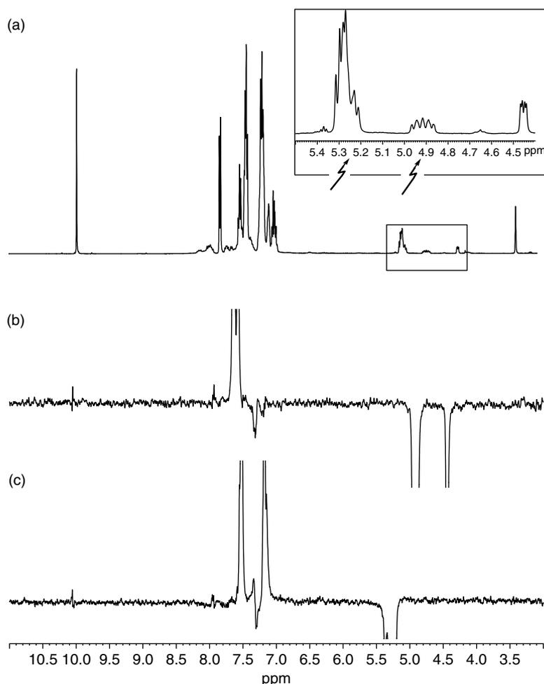
**Figure 5.** (a)  $^1\text{H}$  NMR spectra, 0.5 M THF- $d_8$ , 253 K; the oxaphosphetane protons were irradiated as shown; in (b) (*E*)-oxaphosphetane and (c) (*Z*)-oxaphosphetane. DPGSE-ROE spectra were recorded at 253 K, 64 scans, mixing time 1.4 s, lb 2 Hz.
