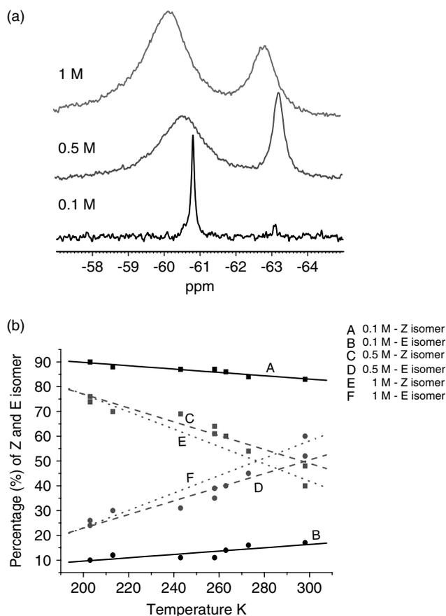
**Figure 2.** (a)  $^{31}\text{P}$  NMR for the Wittig reaction at different reaction concentrations in THF at 203 K; (b) stereochemical drift according to the NMR integration of the oxaphosphetanes.
