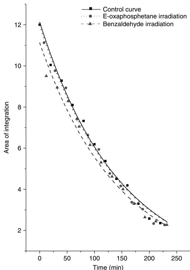
**Figure 4.** Time behaviour of the  $^{13}\text{C}$  NMR signals of the (*Z*)-oxaphosphetane signals during the Wittig reaction at 253 K. The curves show the situation when the spectra was irradiated as a control (at a position where no signal was present) (■) and the situation when the benzaldehyde signal (▲) or the (*E*)-oxaphosphetane (●) was irradiated.
