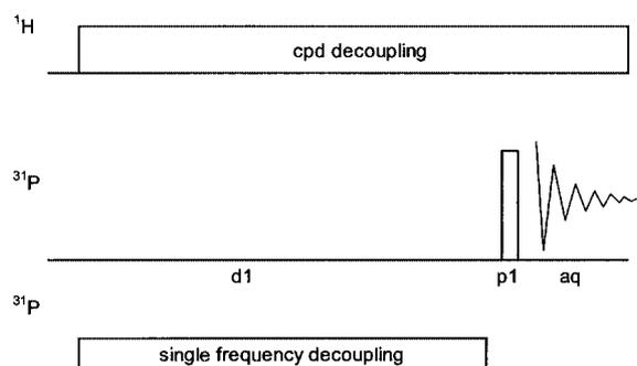
**Figure 1.** Pulse scheme for the saturation transfer experiment with three different r.f. channels, shown for the example of  $^{31}\text{P}$ .
