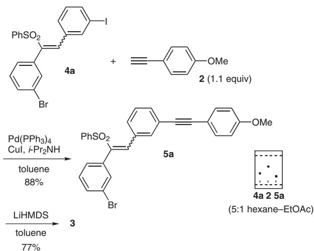
**Scheme 2** Preparation of **3** by use of 1,2-diarylethenyl phenyl sulfone
