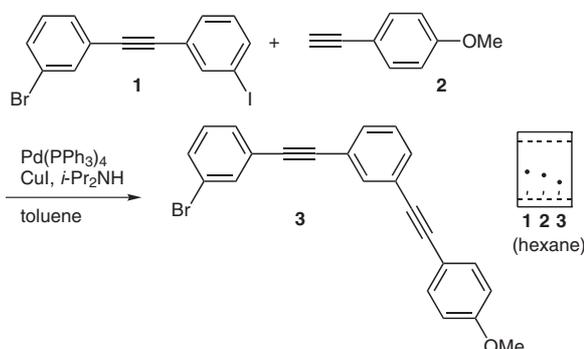
**Scheme 1** Preparation of **3** by use of halogen-substituted diphenylethyne
