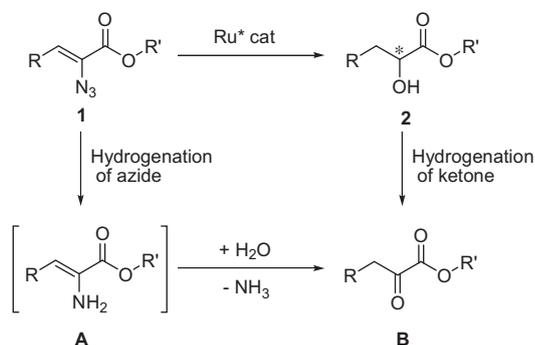
**Scheme 2.** A possible mechanism of asymmetric transfer hydrogenation of  $\alpha$ -azido acrylate.
