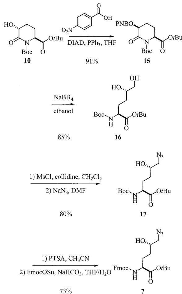
Scheme 2. Synthesis of the (2*S*,5*S*)-5-hydroxyllysine derivative **7**
