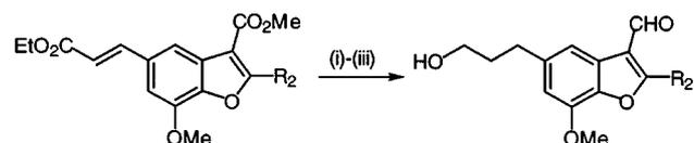
Scheme 3 (i) H<sub>2</sub>, Pd-C, EtOAc; (ii) DiBAL, CH<sub>2</sub>Cl<sub>2</sub>/toluene; (iii) MnO<sub>2</sub>, CHCl<sub>3</sub>
