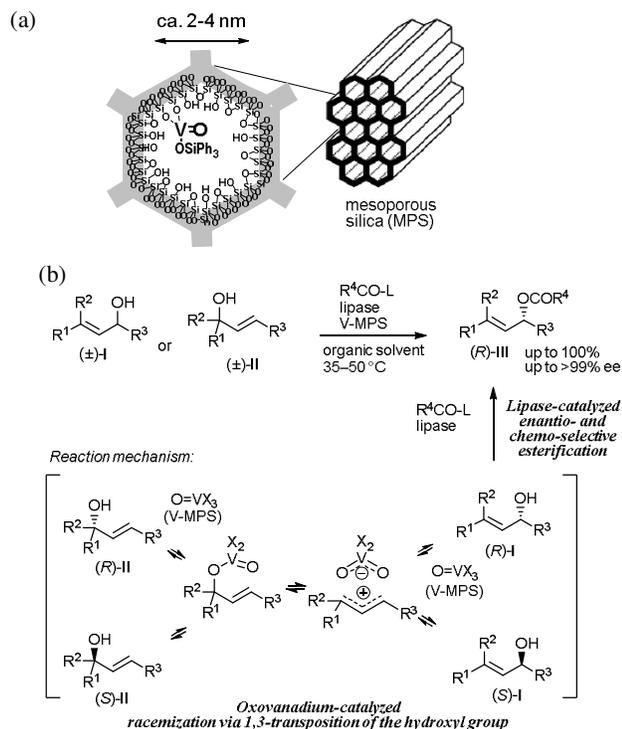
**Fig. 1.** (a) V-MPS structure; (b) Lipase/oxovanadium combo-catalyzed DKR of racemic allylic alcohols (**I** or **II**).
