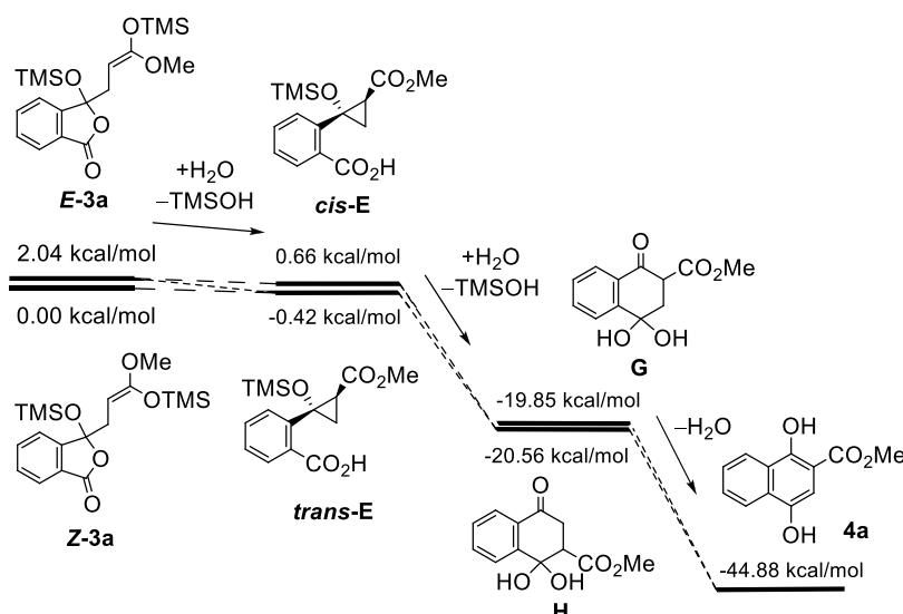
**Scheme 9.** Alternative Presumed Reaction Mechanism of Rearrangement of **3a** to **4a**
