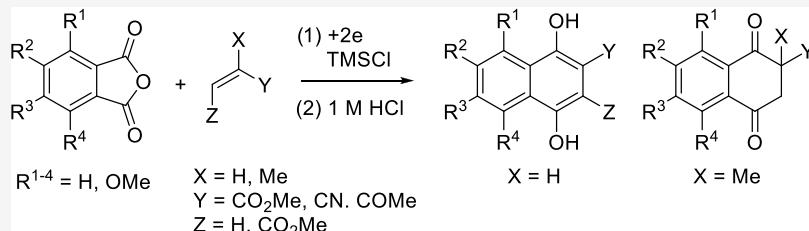
**ABSTRACT:** Electroreductive coupling of phthalic anhydrides with  $\alpha,\beta$ -unsaturated carbonyl compounds in the presence of TMSCl and subsequent treatment with 1 M HCl gave 1,4-dihydroxynaphthalenes and 2-methyl-2,3-dihydronephthalene-1,4-diones.
