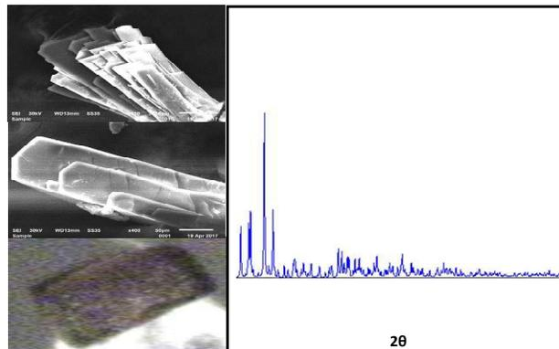
**Figure 5.** SEM micrographs (left panels) and XRPD patterns (right panels) of HCC **3**; (bottom) as synthesised, (middle) before catalysis and (top) after catalysis for the reaction between benzaldehyde and malononitrile.
