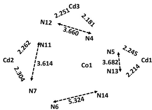
**Figure 3.** A truncated structure of HCC **3** showing various bond distances between Cd(II) ions and separations between two neighbouring nitrogen atoms. The organic framework around the Cd(II) ions and coordinated solvents/ anions are removed for clarity.
