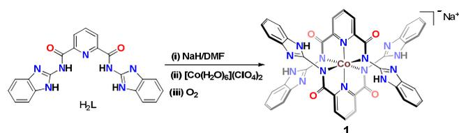
**Scheme 1.** Preparation route for the synthesis of metalloligand **1**.
