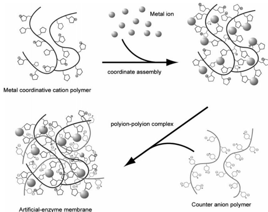
**Figure 2.** Schematic of the synthesis procedure of the artificial enzyme membrane through coordinative self-assembly.
