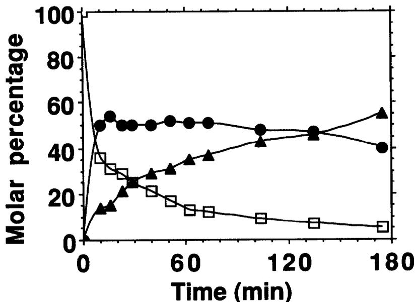
Fig. 3. Course of the S-alkylation of cysteine methyl ester (2.8 equiv) by Br<sub>2</sub>Dmb (2.0 equiv) in DIEA (2.8 equiv) and (CD<sub>3</sub>)<sub>2</sub>SO. The reaction mixture was monitored by proton NMR spectrometry to determine the molar percentages of Br<sub>2</sub>Dmb (squares), an intermediate (circles), and (Cys-OCH<sub>3</sub>)<sub>2</sub>Dmb (triangles) versus time.
