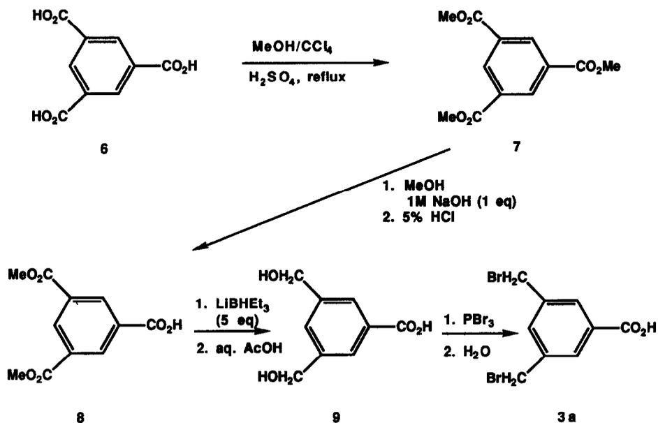
Fig. 2. A regiospecific four-step synthesis of 3,5-bis(bromomethyl)benzoic acid (**3a**) from 1,3,5-benzenetricarboxylic acid (**6**)
