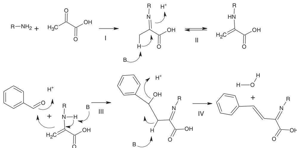
**Fig. 6.** Hypothetical mechanism of the aldol condensation reaction catalyzed by *t*HBP-HA. Schiff base formation (I); imine–enamine equilibrium (II); aldol condensation reaction (III); aldol dehydration (IV).
