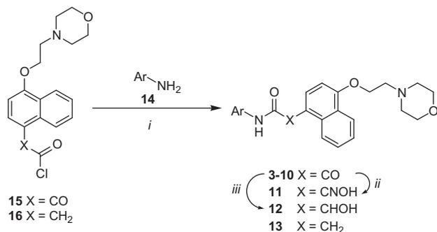
**Scheme 1.** Reagents and conditions: (i) EtOAc, 0.5 N NaHCO<sub>3</sub>, 60 °C, 16 h; (ii) NH<sub>2</sub>OH·HCl, EtOH, pyridine, 45 °C, 12 h; (iii) MeOH, NaBH<sub>4</sub>, rt, 1 h.
