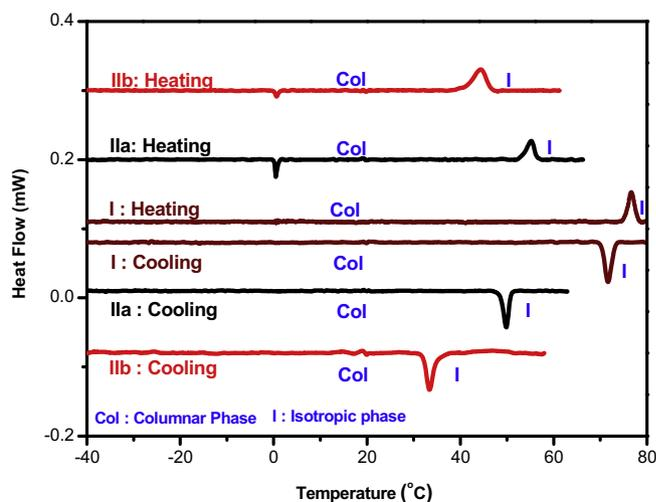
Figure 2. DSC thermograms of mesogens **I** and **IIa–b**.
