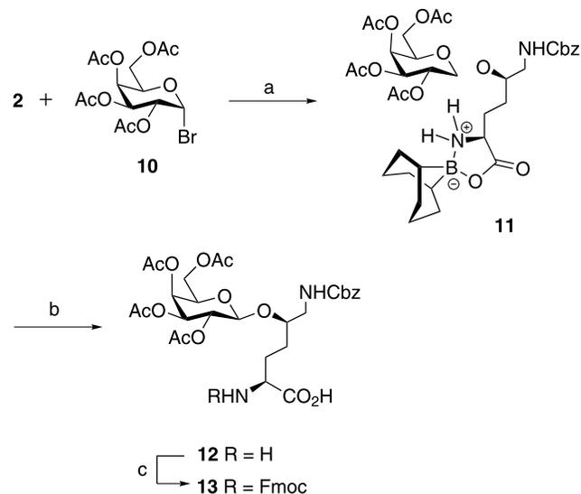
**Scheme 2.** (a) Silver silicate/silver zeolite,  $\text{CH}_2\text{Cl}_2$ ,  $0^\circ\text{C}$ , 8 h (68%); (b)  $\text{CHCl}_3$ –MeOH, rt 12 h; (c) Fmoc-OSu,  $\text{NaHCO}_3$ , acetone– $\text{H}_2\text{O}$  (91% from **11**).
