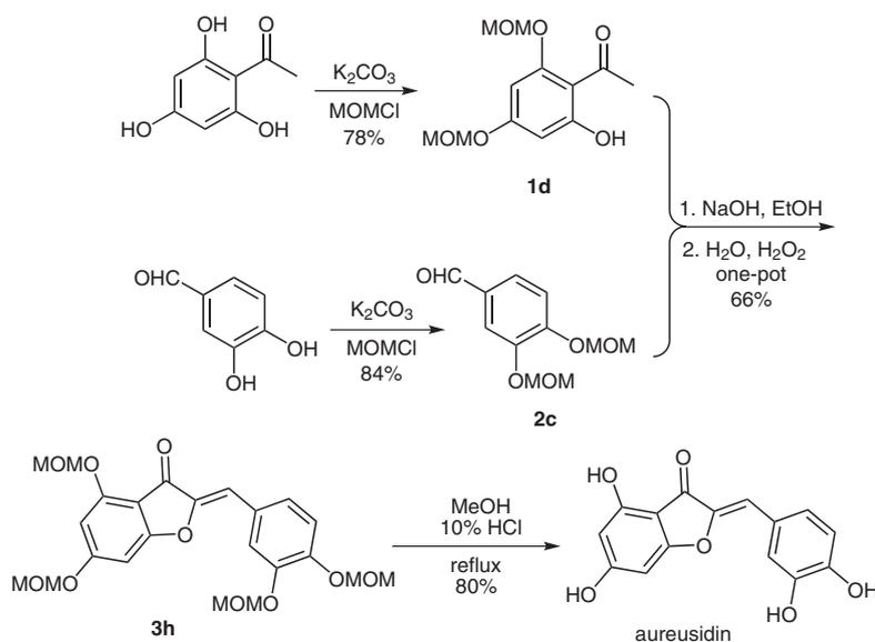
**Scheme 1** Application of the one-pot procedure to the synthesis of aureusidin
