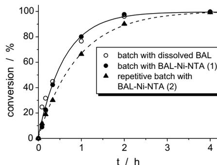
**Figure 1.** Repetitive batch synthesis of (*R*)-2-hydroxy-1-phenyl-propanone with immobilized benzaldehyde lyase (BAL-Ni-NTA) in KPG-stirred tank reactors (10mg BAL [(1) and (2): 10mg BAL on 1mL Ni-NTA-Superflow], 50mM triethanolamine buffer, pH = 8, 0.5mM ThDP, 0.5mM  $\text{MgSO}_4$ , 30vol% DMSO, 10mM benzaldehyde, 60mM acetaldehyde).
