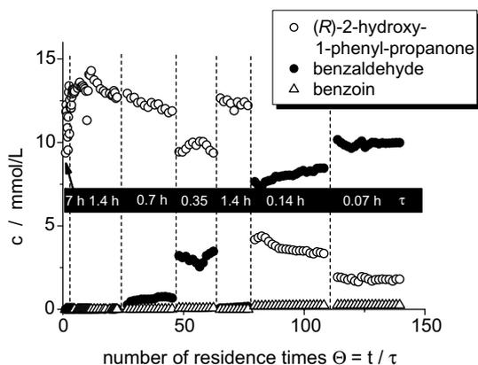
**Figure 2.** Continuous synthesis of (*R*)-2-hydroxy-1-phenyl-propanone in a plug flow reactor, the residence time is indicated in the graphic (50 mg BAL on 5 mL Ni-NTA-Superflow, 50 mM triethanolamine buffer, pH = 8, 0.5 mM ThDP, 0.5 mM MgSO<sub>4</sub>, 30 vol% DMSO, 13 mM benzaldehyde, 60 mM acetaldehyde).
