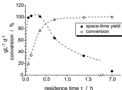
**Figure 3.** Space-time yield and conversion depending on the average residence time in the plug flow reactor. The data points correspond to the mean values obtained at different residence times and displayed in Figure 2. Dashed lines (---) are only drawn as visual aids.
